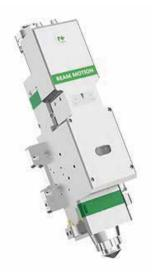
The cutting head has built-in motor drive unit through the linear driver and the focusing lens can automatically change the position in the range of 22mm. The user can set the focus continuously through the program to complete the rapid piercing of thick sheets or other different thickness and materials
